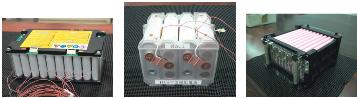
(a) 240 Wh-class battery module • Ni-Mn-Co oxide cathode • 6.8 Ah x 10 cells (b) 260 Wh-class battery module • Mn oxide cathode • 18.4 Ah x 4 cells (c) 260 Wh-class battery module • Ni oxide cathode • 7.2 Ah x 10 cells
