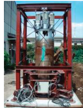
Fig.2 In Situ Triaxial Rock Mass Test System Developed by the Laboratory
