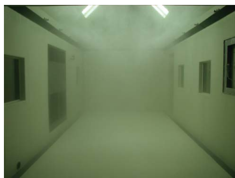
An inside view of the environmental load simulator during salt water spraying
