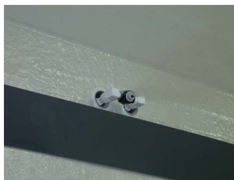
Salt water mist nozzle of the environmental load simulator
