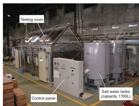
Entire view of the environmental load simulator
