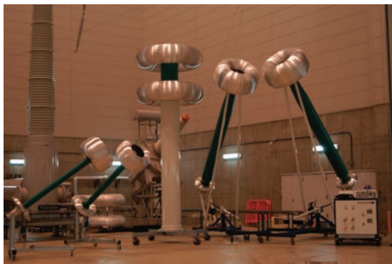
Standard capacitor and water termination system for voltage withstand test of EHV and UHV class XLPE cable system
