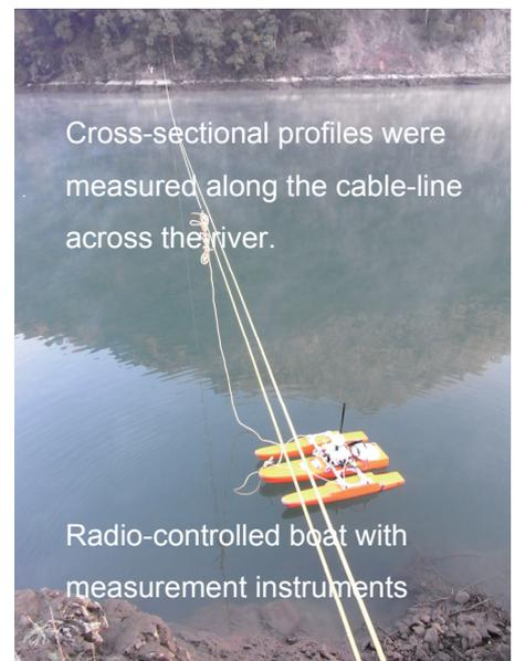
**Fig. 4 Movable current measuring system**
