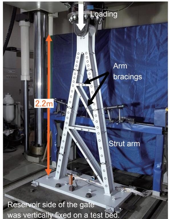
**Fig. 2 Loading test of dam gate model**
