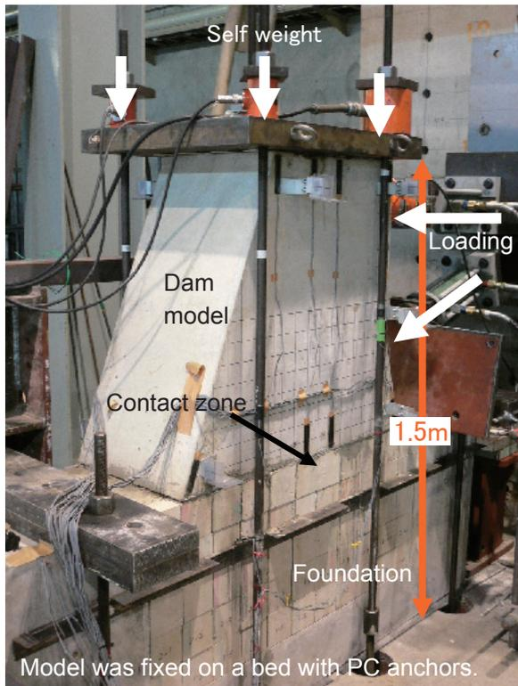
**Fig. 1 Loading test of concrete gravity dam model**
