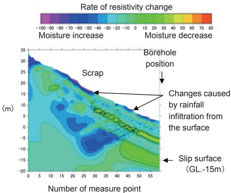
**Fig. 3 Visualization example of soil-moisture distribution**
