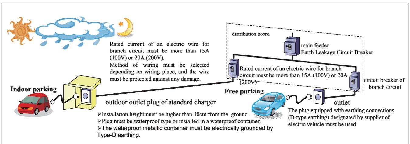
**Fig.3** Example of installation of standard charger
