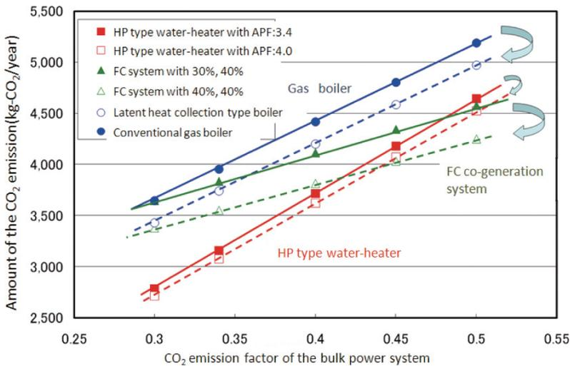
**Fig. 2** Comparison of CO<sub>2</sub> emissions from residential houses installed with high efficiency water-heater systems with consideration given to residential demands.
