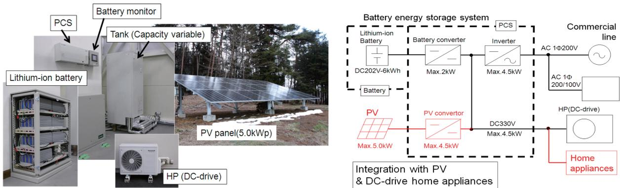
**Fig.1** Plot type battery energy storage system integrated with heat pump water heater for residential use connected with PV (left: components, right: system diagram), for validation of energy efficiency improvement under the simulated conditions with daily heat-water demand pattern in a house, and propose of operation method for absorption of excess energy generated by PV.
