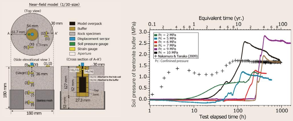
Fig. 3: Prediction experiment of long-term behavior in the near-field using the "CENTURY5000-THM" centrifuge (left: near-field model of this study, right: time-dependent change of the soil pressure of the bentonite buffer through the difference of the boundary condition)
