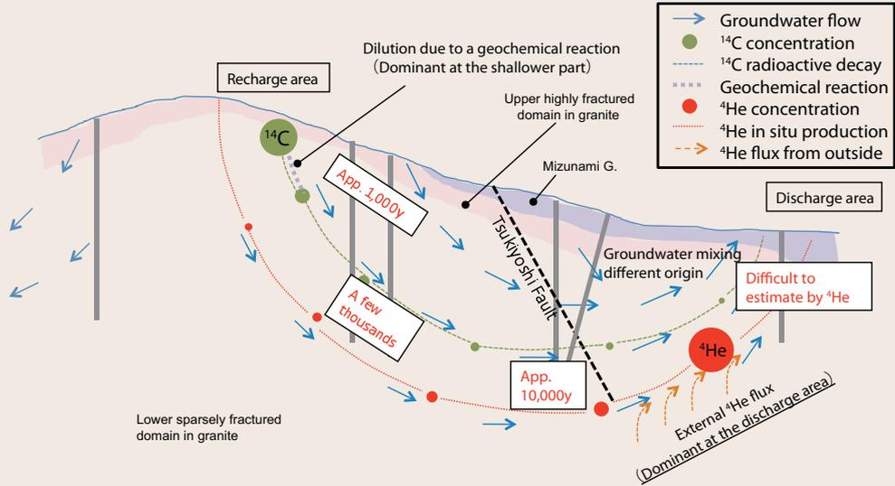
Fig. 1: Conceptual transport model of <sup>14</sup>C and <sup>4</sup>He for groundwater dating in the Tono area
