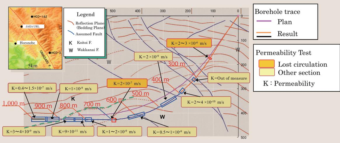
Fig. 2: Results of controlled drilling and the permeability test in the borehole
