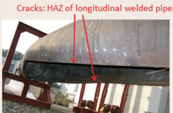
Fig. 5: Photograph of a ruptured 9Cr steel pipe with the dimensions of the actual equipment (Temperature, 650°C; rupture time, approximately 8,600 h)
