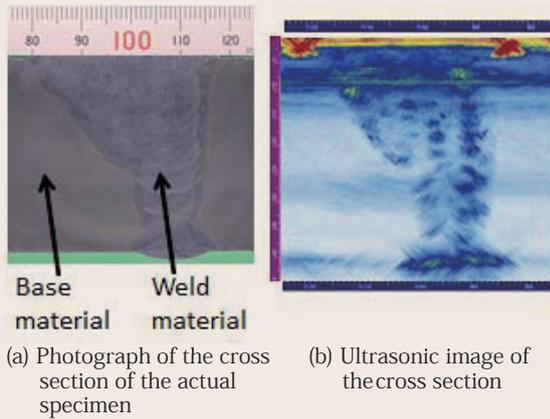
Fig. 1: Estimation of the shape of weld metal
