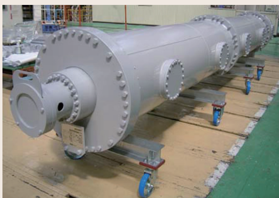
Fig. 5: Container including a prototype 300 kV-class gas/solid hybrid insulated bus model
