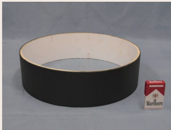
Fig. 2: Prototype large cylinder of \phi 450 mm in diameter
