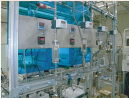
The Cs adsorption performance of the single-column test and the series-column test, simulated for an actual system, can be evaluated by opening or closing the valve in this system.
