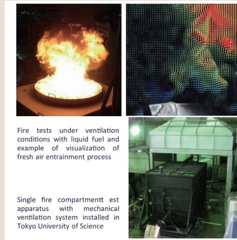
Fig. 2: Heat source characteristics of liquid fuel in a compartment under ventilation conditions
