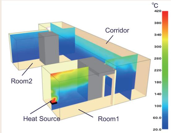
Fig. 1: Example of simulation of multi-room fires using a fire model FDS
