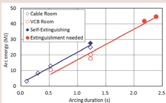
Fig. 3: Ignition conditions between arcing energy and duration measured in the HEAF tests using high-voltage metal-clad switchgears
