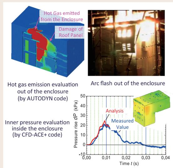
Fig. 4: Estimation of internal pressure and hot gas emission from the damaged enclosure
