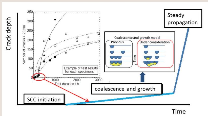
**Fig. 2: Time dependence of crack depth (greater than 20 micrometers) for low-carbon stainless steel**
