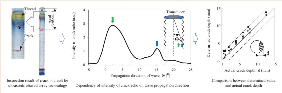
**Fig. 1: Inspection and sizing method of cracks for embedded foundation bolts**
