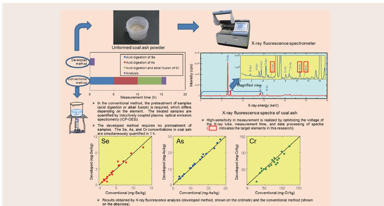
**Fig. 1: Simple and rapid quantification of Se, As, and Cr concentrations in coal ash**
