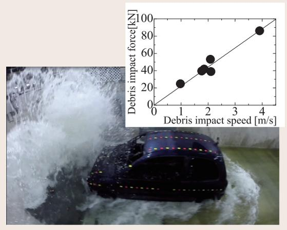
Fig. 4: Evaluation of tsunami-debris impact force
