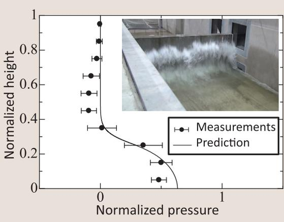
Fig. 3: Evaluation of tsunami impact pressure
