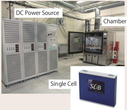
Fig. 1: Lithium-ion cell and charge-discharge test equipment used in this study
