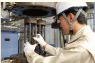
Crack propagation testing for structural materials for nuclear reactors
