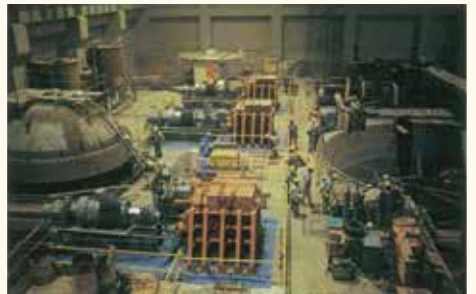
Forced vibration test inside nuclear power plant building
