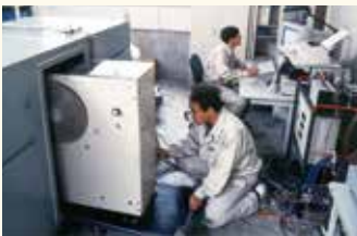
Performance evaluation testing for prototype of CO 2 heat pump
