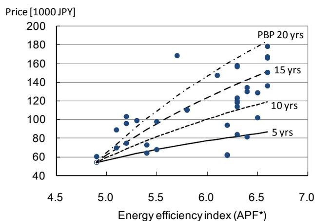
**Figure 7. Price, energy efficiency, and payback periods of room air conditioners (2.8 kW class) in 2006**
