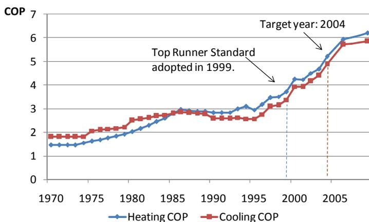
**Figure 3. Long term trend of energy efficiency of room air conditioners**
